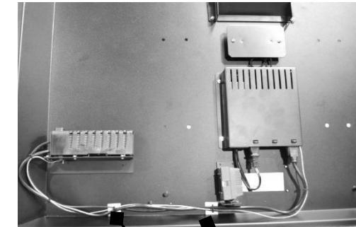
Use Wire tie holders included to secure wire tied cables stay in place
