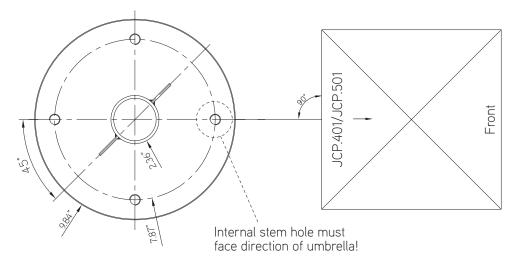
Dig an approximate 90cm/3ft. deep by 60cm/2ft. wide hole. Insert in-ground fitting and pour mixed concrete into hole around fitting. Make sure in-ground plate is level.
