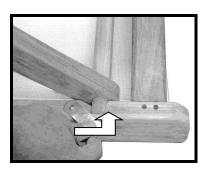
**STEP-I**Carefully lift the LEG ASSEMBLY as shown in the photograph. Fit opposing dowel rod into position as shown and lock the LEG ASSEMBLY into place.
