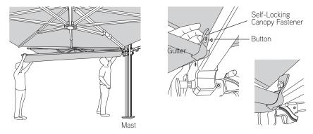
3. Attach other end of gutter (velcro end) to button located near both rib ends. Repeat step 2-3 as necessary (depending on number of gutters installing).
