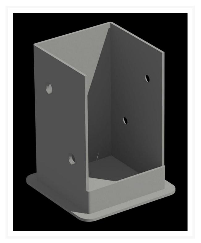
The Bolt Down Bracket System enables pergola owners to mount their pergola safely and securely to a wood deck or cement patio. Simply bolt the galvanized steel brackets into place. Insert 4x4 pressure treated wood posts (purchased separately) into the brackets and screw them in place. Slide your pergola posts over the wood posts and screw the pergola posts into the wood.
