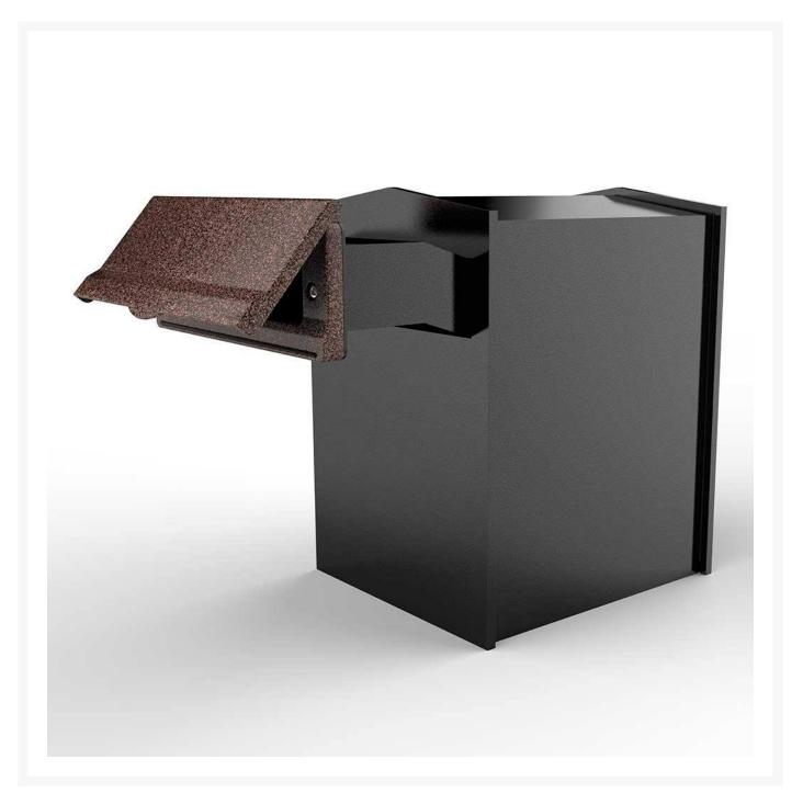
Mounted through a wall, mail is delivered through a conventional letter plate. The mail then passes through a chute, drops into a collection box and is retrieved from the rear lockable secure access door. Choose an adjustable chute depth of 4" to 6" inches or 8" to 10" inches to match the thickness of your wall. The chute is held in place with masonry and silicone adhesive. (not provided) Mailbox is made from solid aluminum, is
